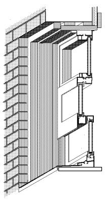
UNACCEPTABLE ALUMINUM REPLACEMENT WINDOWS Even though this window's proportions approximate those of the wooden window, the framing members have almost no depth and there is almost no setback between the glass and the sash.
